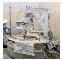
In addition to the requirements from UL and the FDA, cables in food and beverage applications must be able to withstand repeated washdown with a wide variety of chemicals. If a cable cannot withstand frequent washdown cycles, the cable jacket may become degraded. A damaged cable jacket can quickly lead to cable failure and may pose a safety hazard. For this reason, cables for the food and beverage industry should be certified for washdown resistance.
