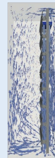
Circulation flow around the AirSTREAM frame with a fitted AirBLOWER fan system
