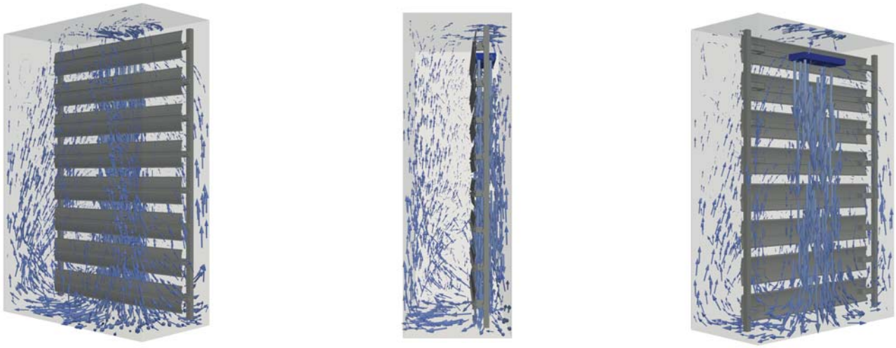
Figure 1: Circulation flow around the AirSTREAM frame with a fitted AirBLOWER fan system
