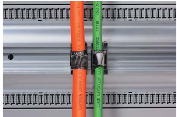
EMC snap on accessory for the DIN rail profiles. This can be simply positioned on a DIN rail. Shielded cables can be fitted directly in front of the part using shield clamps or spring shield clamps.
