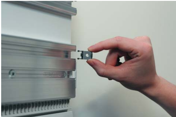
Step 1: Sliding nut pieces (with thread M3-M8) can be simply slipped into the sliding nut channel with a sliding nut cage.
