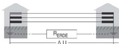
Potential differences due to earth loops
